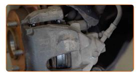
Install the brake caliper retaining spring.
