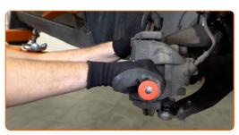
Clean the brake caliper bracket fasteners. Use a wire brush. Treat the brake caliper bracket fasteners. Use WD-40 spray.
