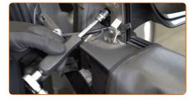
Attach the mirror adjuster connector to the door.
