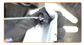
Attach the ABS sensor connector.
