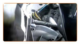
5 Detach the accelerator pedal connector.
