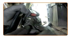
6 Remove the accelerator pedal.
