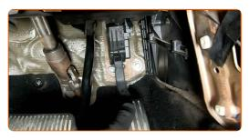
Return the accelerator pedal to its initial position and screw in its fastener. Use a drive socket #10. Use a ratchet wrench.
