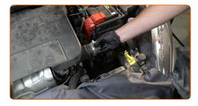
Reinstall the air filter housing.
