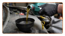
Replacement: engine oil and filter – FORD Focus Mk2 Box Body / Estate.
