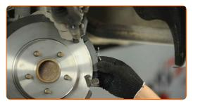
Replacement: brake pads - FORD Focus Mk2 Box Body / Estate. Tip:
