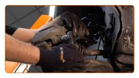
Remove the brake caliper.
