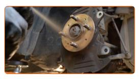
20 Install the brake disc.
