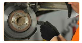
18 Remove the brake disc.
