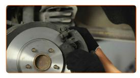
Clean the brake caliper guide pins.
