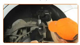
Install the brake caliper and fix it.
