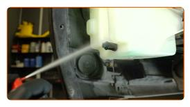
19 Install a new washer pump seal.
