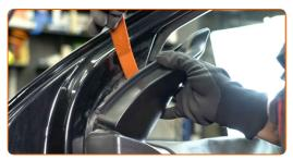
Disconnect the wiring of the wing mirror. Use a clip removal tool.
