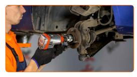
Remove the drive shaft. Use a hammer.
