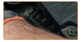
Remove the air intake pipe.
