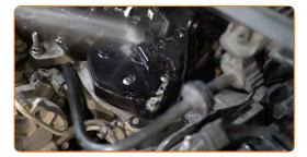
Screw the fixing bolts of the fuel filter bracket. Use a drive socket #8. Use a ratchet wrench.
