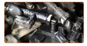
Connect the bleeder kit to the fuel filter bleeder screw.
