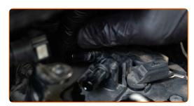
Loosen the fuel filter mounting. Use a drive socket #8. Use a ratchet wrench.
