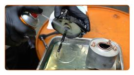
Install and tighten the cap of the fuel filter housing. Use Torx T15. Use a ratchet wrench.
