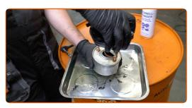
Clean the fuel filter housing and the cover. Use all-purpose cleaning spray.
