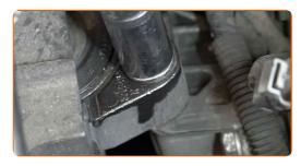
Clean the engine mount fasteners. Use a wire brush. Use WD-40 spray.
