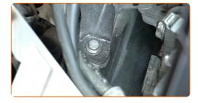
Unscrew the fasteners that connect the engine mount to the car body. Use a drive socket #18. Use a ratchet wrench.
