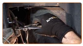
Loosen the brake hose fastening. Use a flare nut spanner #14.
