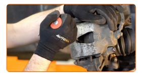
16 Remove the brake caliper.
