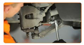
Remove the guide pins from the brake caliper.
