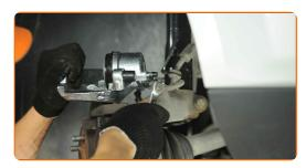
Remove the brake hose clamp.
