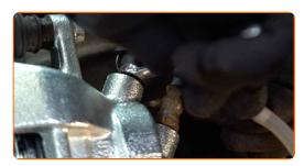
Bleed the brake caliper system. Without starting the engine, press the brake pedal several times until you feel significant resistance.
