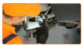
Clean the brake caliper surface.
