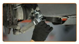
Clean the brake caliper guide pins.
