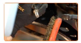
Treat the mounting seats of the tie rod end. Use copper grease.
