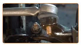
Tighten the fastening nut connecting the tie rod end to the steering knuckle. Use a drive socket #15. Use a torque wrench. Tighten it to 48 nm torque.
