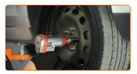
Lower the car and working in a cross order, tighten the wheel bolts. Use wheel impact socket #19. Use a torque wrench. Tighten it to 120 nm torque.
