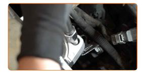
Tighten the fasteners that connect the engine mount to the car body. Use a drive socket #18. Use a torque wrench. Tighten it to 65 Nm torque.
