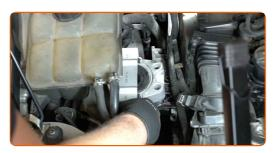
Tighten the engine mount fastening bolts. Use a drive socket #E11. Use a torque wrench. Tighten it to 32 Nm torque.
