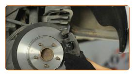
Clean the brake caliper guide pins.
