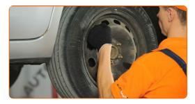
Detach the brake caliper retaining spring. Use a flat screwdriver.
