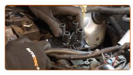
Tighten the ignition coil fastening. Use Torx T20. Use a torque wrench. Tighten it to 8 nm torque.
