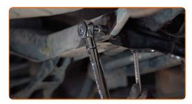
Tighten the fasteners connecting the control arm to the rear knuckle. Use a drive socket #18. Use a torque wrench. Tighten it to 115 Nm torque.
