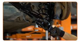
Screw in the fasteners connecting the control arm to the rear knuckle. Use a drive socket #16. Use a ratchet wrench.
