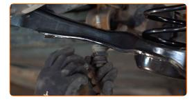
Tighten the stabiliser link fastener. Use a combination spanner #15. Use a drive socket #15. Use a torque wrench. Tighten it to 15 Nm torque.
