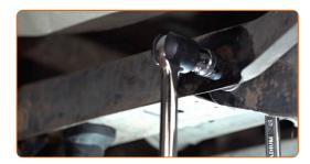
Unscrew the fastener connecting the control arm to the rear knuckle. Use a drive socket #16. Use a ratchet wrench. Remove the fastening bolt.
