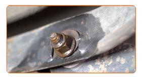
Unscrew the arm fastening to the beam. Use a drive socket #18. Use a combination spanner #19. Use a tap wrench.
