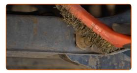
Unscrew the stabilizer rod fasteners. Use a combination spanner #15. Use a drive socket #15. Use a ratchet wrench.
