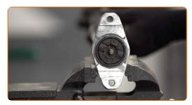
Fix the shock absorber mount. Use a combination spanner #13. Use a drive socket #13. Use a torque wrench. Use an adjustable wrench. Tighten it to 25 Nm torque.
