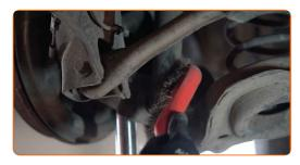
Unscrew the lower fastener of the shock absorber. Use a drive socket #16. Use a ratchet wrench. Use a tap wrench.
