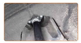
Remove the support from under the rear arm.
