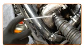
Loosen the binding clamps attaching the air duct to the air filter housing and to the charger. Use a drive socket #7. Use a ratchet wrench.
