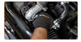
Tighten the binding clamps that attach the air duct to the air filter housing and to the charger. Use a drive socket #7. Use a ratchet wrench.
