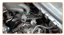
Unscrew the fuel filter bracket. Use a drive socket #E11. Use a ratchet wrench.
