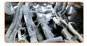
Install the EGR valve hose clamp. Use clic-R collar pliers.
