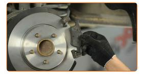
Replacement: brake pads – FORD Focus II Hatchback (DA\_, HCP, DP). Tip from AUTODOC:
