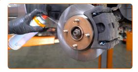
Replacement: brake pads – FORD Focus II Hatchback (DA\_, HCP, DP).
