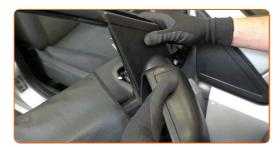
Tighten the screws of the wing mirror. Use Torx T25. Use a drive socket #10. Use a torque wrench. Tighten it to 5 Nm torque.
