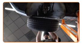
Disconnect the wiring and the brake hose from the bracket on the shock strut.
