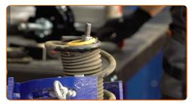
Release the coil spring.
