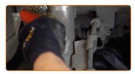
Unscrew the nut and remove the stabilizer rod from the shock strut. Use a drive socket #15. Use a ratchet wrench.
