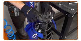
Tighten the shock strut piston rod nut. Use Torx T30. Use a combination spanner #19. Use a torque wrench. Tighten it to 50 Nm torque.
