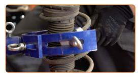
Remove the strut piston rod nut. Use Torx T40. Use a combination spanner #19. Use a ratchet wrench.
