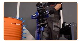
Remove the assembled shock strut.
