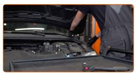
Unscrew the fasteners of the windscreen wiper arms. Use a drive socket #15. Use a ratchet wrench.
