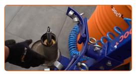
Install the spring on the shock absorber.
