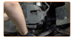
Unscrew the upper fastening of the shock absorber strut.
