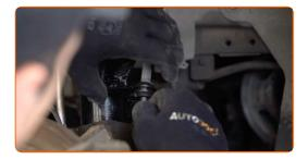
Secure the stabilizer link on the suspension strut. Use a drive socket #15. Use a torque wrench. Tighten it to 48 Nm torque.
