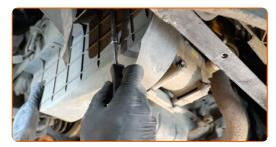
Tighten the fasteners of the oil pan lower cover. Use Torx T30. Use a ratchet wrench.
