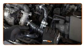
On the right side, attach the PCV valve hose to the engine cover.
