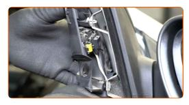
Screw in the fasteners of the wing mirror trim panel. Use Torx T25.
