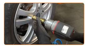
Lower the car and working in a cross order, tighten the wheel bolts. Use wheel impact socket #19. Use a torque wrench. Tighten it to 120 Nm torque.
