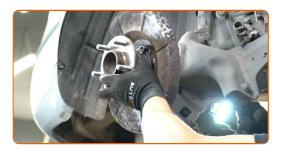
Remove the brake disc baffle plate.
