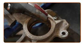
Install the new wheel hub with a bearing. Use a bush and bearing driver set.
