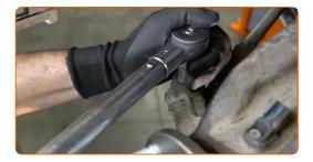
Tighten the ball joint fastener. Use a combination spanner #21. Use a torque wrench. Tighten it to 70 Nm torque.
