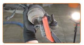
Clean the fasteners connecting the shock strut to the steering knuckle. Clean the fastener connecting the ball joint to the steering knuckle. Use a wire brush. Use WD-40 spray.
