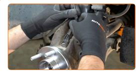
Install and tighten the drive shaft bolt. Use a drive socket #12. Use a ratchet wrench.
