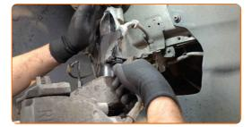
Clean the mounting seats of the stabiliser link. Use a wire brush. Use WD-40 spray.
