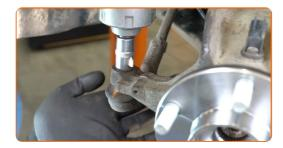
Tighten the fastening nut connecting the tie rod end to the steering knuckle. Use a drive socket #15. Use a torque wrench. Tighten it to 48 Nm torque.
