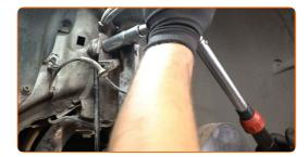
Treat the shock strut fasteners. Treat the fastener connecting the tie rod end to the steering knuckle. Treat the fasteners of the ball joint. Use copper grease.
