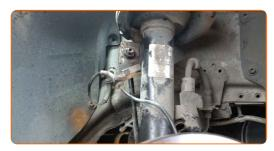
Tighten the fastener connecting the stabilizer link to the shock strut. Use a drive socket #17. Use a torque wrench. Tighten it to 48 Nm torque.
