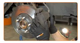
Tighten the brake caliper bracket. Use a drive socket #15. Use a torque wrench. Tighten it to 90 Nm torque.
