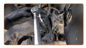
Attach the ABS sensor connector.
