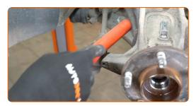
Unscrew the end fastening nut to the steering knuckle. Use a drive socket #15. Use a ratchet wrench.
