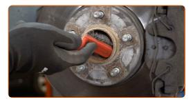
Loosen the fastener of the driveshaft. Use a drive socket #12. Use a tap wrench.
