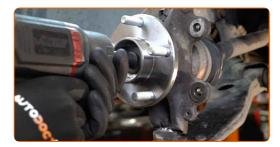
Clean the hub. Treat the contacting surface. Use copper grease.
