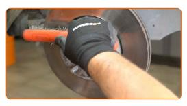
21 Remove the brake disc.
