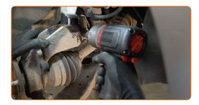
Remove the fastening bolt.
