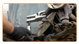
Clean the fasteners connecting the shock strut to the steering knuckle. Use a wire brush. Use WD-40 spray.
