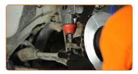
Tighten the tie rod end locknut. Use a combination spanner #24. Use a torque wrench. Tighten it to 62 nm torque.
