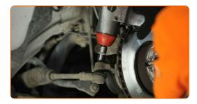
Disconnect the tie rod end from the steering knuckle. Use a ball joint puller.
