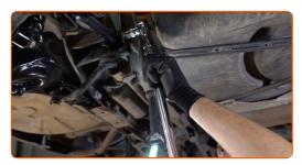
Tighten the fasteners connecting the control arm to the rear knuckle. Use a drive socket #15. Use a torque wrench. Tighten it to 115 Nm torque.
