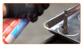
Treat the brake caliper guide pins. Use the brake caliper guide pin grease.
