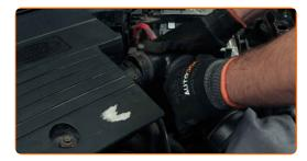
Detach the air intake hose clamp. Use clic-R collar pliers.
