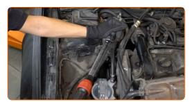
Tighten the fasteners that connect the engine mount to the car body. Use a drive socket #16. Use a torque wrench. Tighten it to 57 Nm torque.
