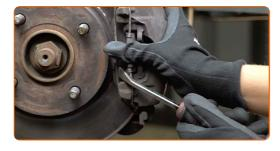
Remove the brake caliper.
