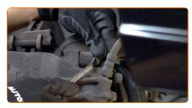
Clean the brake caliper fasteners. Use a nylon cleaning brush. Use a brake cleaner.
