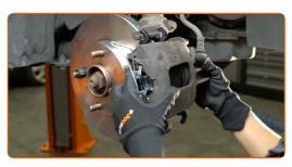
20 Install the brake caliper retaining spring.
