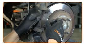
Clean the brake caliper bracket fasteners. Use a wire brush. Use WD-40 spray.
