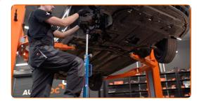
Install and tighten a new bolt of the steering knuckle. Use a drive socket #18. Use a ratchet wrench. Use a torque wrench. Tighten it to 90 Nm torque.
