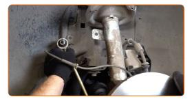
Unscrew the lower fastener connecting the shock strut to the steering knuckle. Use a drive socket #18. Use a ratchet wrench. Use a tap wrench.
