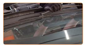
Tighten the fasteners of the wiper arms. Use a drive socket #15. Use a torque wrench. Tighten it to 10 Nm torque.
