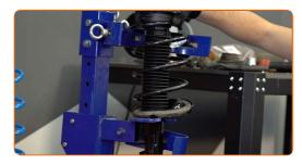
Clean the mounting seats of the shock strut. Use a wire brush. Use WD-40 spray.
