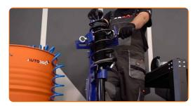
Remove the assembled shock strut.
