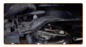
Install the fasteners of the wiper plastic cowl grille.
