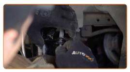
Secure the stabilizer link on the suspension strut. Use a drive socket #15. Use a torque wrench. Tighten it to 48 Nm torque.
