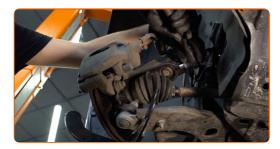
Disconnect the steering knuckle from the shock absorber strut. Use a crowbar.
