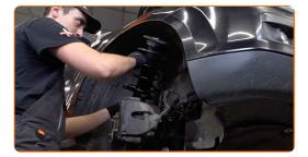
Secure the upper fasteners of the shock strut (3 pieces). Do not tighten it.
