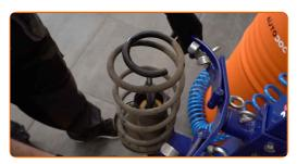
Install a new shock strut mount and tighten it.
