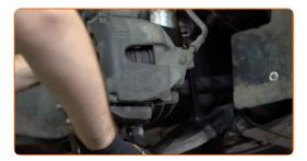
Unscrew the upper fastening of the shock absorber strut.
