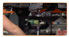
Release the lower fastener connecting the shock strut to the steering knuckle. Use a special drive socket to remove the shock absorber. Use a hammer. Use a flat metal-working chisel.
