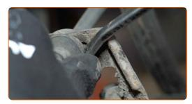
Remove the brake caliper together with its bracket. Use a crowbar.
