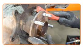
Clean the ABS sensor mounting seat. Use all-purpose cleaning spray.
