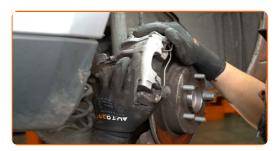
Tighten the brake caliper bracket. Use a drive socket #13. Use a torque wrench. Tighten it to 55 Nm torque.
