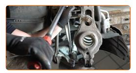
Treat the ABS sensor connector. Use electronic spray.
