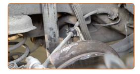
Install the parking brake cable into the brake caliper bracket. Use water pump pliers.
