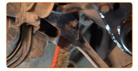
Unscrew the arm fastening to the beam. Use a drive socket #15. Use a ratchet wrench. Use a tap wrench. Remove the fastening bolt.
