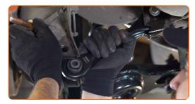
Install the control arm fasteners. Use a crowbar.
