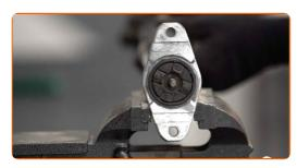
Screw the shock strut piston rod upper fastening. Use a combination spanner #13. Use a drive socket #13. Use an adjustable wrench. Use a torque wrench. Tighten it to 25 Nm torque.
