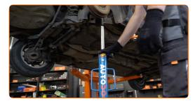
Clean the fasteners of the shock absorber upper mount. Use a wire brush. Use WD-40 spray.
