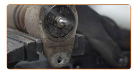
Remove the shock absorber piston rod fastening. Use a combination spanner #13.
