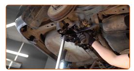
Tighten the shock absorber mount fasteners. Use a drive socket #10. Use a torque wrench. Tighten it to 25 Nm torque.
