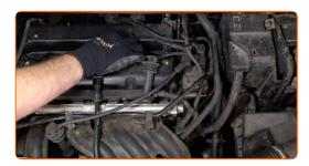
Screw new spark plugs and tighten them. Use the spark plug socket #16. Use a torque wrench. Tighten it to 15 nm torque.
