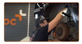
Install the shock absorber mount using the center hole as a guide.
