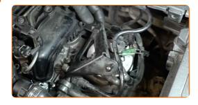
Screw the fixing bolts of the fuel filter bracket. Use a drive socket #10. Use a ratchet wrench.
