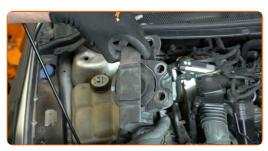
Replacement: engine mounts – FORD Focus C-Max (DM2). Tip from AUTODOC:
