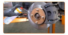
Replacement: brake pads – FORD Focus C-Max (DM2). AUTODOC recommends:
